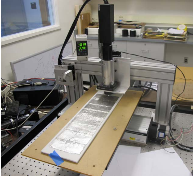
Figure 10: View of the 1878 St. Louis Edison Tinfoil being scanned with the confocal probe in Berkeley in 2012. The probe performed a raster sweep in order to cover the entire foil.
