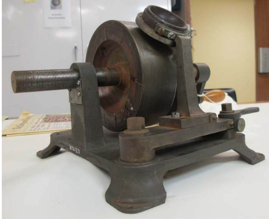
Figure 11: The 1881 Bell Graphophone, an Edison tinfoil machine which has been coated with wax as an experimental recording medium.
