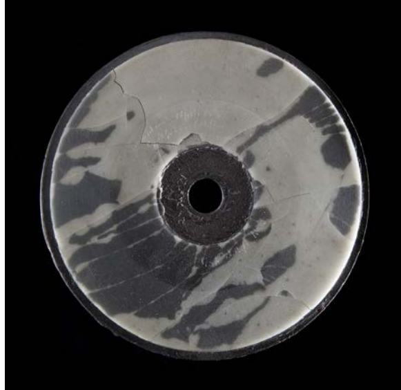
Figure 13: Wax on binder board disc from the Smithsonian Volta Laboratory collection which contains a recording of Alexander Graham Bell.
