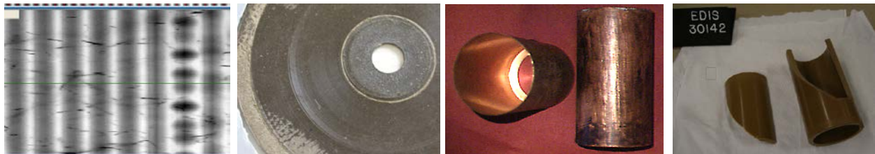
Figure 7: From the left (a) Greyscale (depth) image from Hearst Museum wax cylinder showing clear damage from fibers on the surface (~1910). (b) Example of experimental Bell recording, wax on paper, from the Smithsonian (early 1880's) (c) Example of copper cylinder galvano mold from the Berlin Phonogramm Archive (early 20th century). (d) The Dickson Cylinder from the Edison National Historic Site, first film soundtrack experiment (1893).
